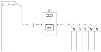
The control panel shall incorporate five large, green," illuminated LED displays, for the Left Bank, the Right Bank, Delivery Pressure, Intermediate Pressure and Emergency Reserve Bank Pressure.
