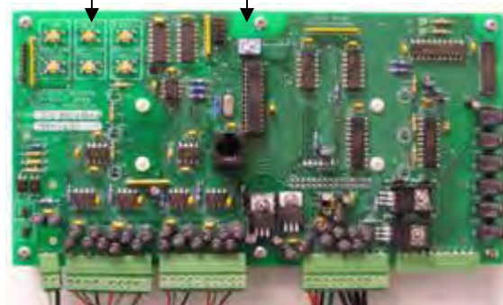
Dip switch #1 RUN/PROGRAM
